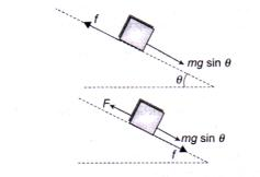
Component of weight along inclined plane + force of friction =  $2mg \sin \theta$
