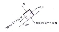
$f_{\rm lm} = \mu N = 0.7 \times 80 = 56 \text{ N}$ Net driving force = 60 - 40 = 20 N (down the plane) As resisting force is greater than net driving force, the friction will be static of nature and friction force is 20 N (up the plane).
